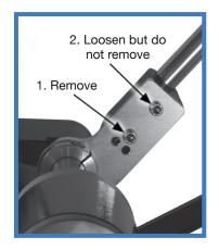
**First**, on the inside of the base of each lever, use your 5mm Hex Key loosen the top screw but do not remove it. Remove the bottom screw. Keep the washers on the screw.
