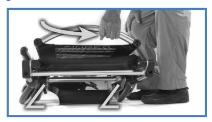
There are many occasions in which you will need to lay the Zinger on the floor. First fold the Zinger as described on the previous page. Next lower the Seat Back Bar until the Front Caster Wheels begin to contact the ground. At this point apply a rotational motion (top arrow) as you lower it further, so that the Front Caster Wheels both lie down together in the same direction. If you do not use this rotational motion the caster wheels may stand up thus preventing the Zinger from lying flat.
