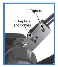
**To adjust lever lower**, drop the lever so that the lower screw can be threaded into the hole as shown. Be absolutely certain to tighten both screws firmly.
