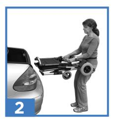
Next, grab the Cross Tube to lift the Zinger off the ground with the Battery cradle pressed against your thighs.
