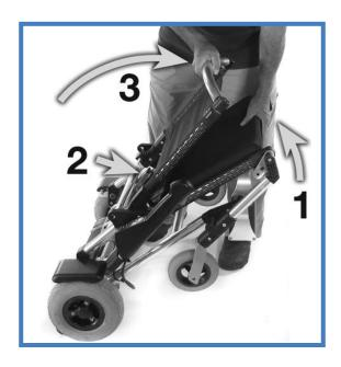
**NOTE:** The parking brakes should automatically set each time the Zinger is unfolded, but always double check before sitting.
