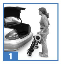
Grab the Anti-Tip Wheels and lift the rear of the Zinger so that it leans against your upper thighs as shown.
