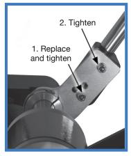
**To adjust lever higher**, lift the lever so that the bottom screw can be threaded into the hole as shown. Be absolutely certain to tighten both screws firmly.
