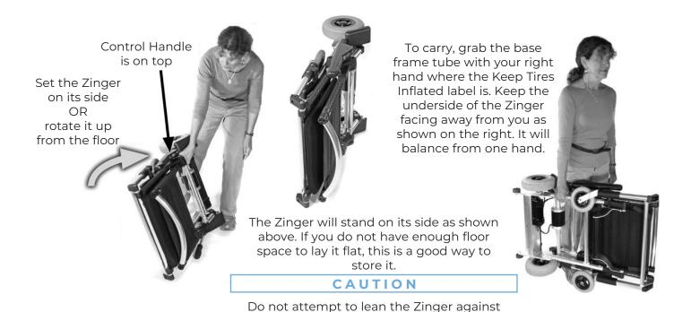
a wall on its rear Anti-Tip Wheels. It will roll out from the wall.
